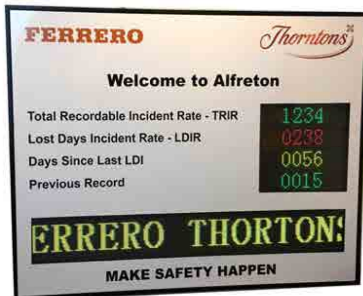
Below and Right: A similar layout on these Health and Safety Displays for Berkeley and Ferrero Thorntons, but the 64 x 64 pixels LED panel is used to display 4 lines but with a smaller text height. A smaller information screen is at the bottom for general information.
