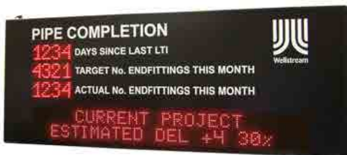
Below: 3 row 4 digit counter display with MS24/80-2L red LED internal display used in a factory production environment. This sign doubles up to show health & safety related information in the 2 line display beneath.
