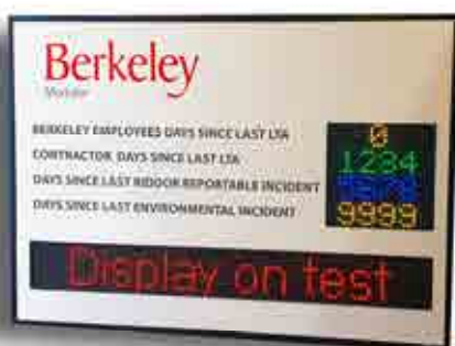
Below and Right: A similar layout on these Health and Safety Displays for Berkeley and Ferrero Thorntons, but the 64 x 64 pixels LED panel is used to display 4 lines but with a smaller text height. A smaller information screen is at the bottom for general information.
