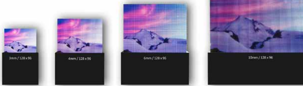
These LED screens have the same screen resolution but with different LED pitches, they are different sizes. Viewed at 4 metres, so only the 3mm and 4mm look crisp.
