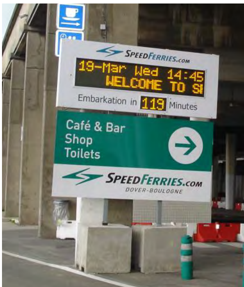
Below: Two line 16 character information display with countdown timer to show minutes to embarkation at a ferry terminal
