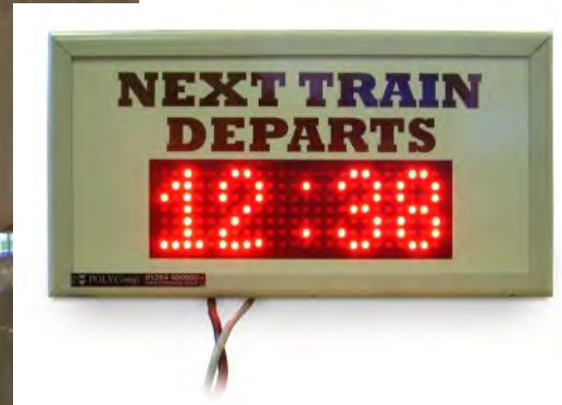
Below: MS24/60-3L display showing passenger information and train times
