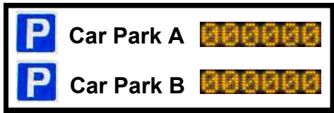
Two 6 character LED panels with static text
