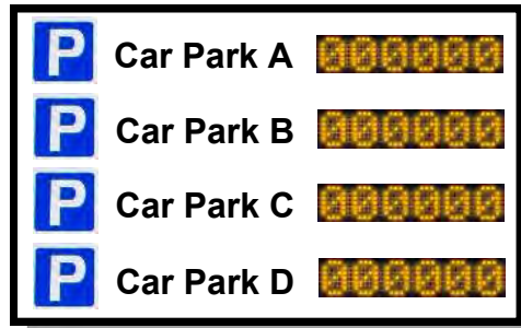
Four 6 character LED panels with static text
