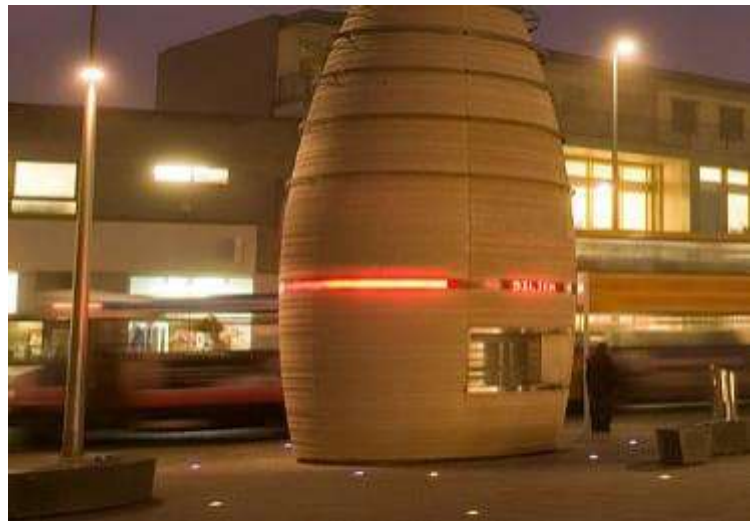
Above: 60mm character height continuous single line display around a ticket booth in Western Supermare.
