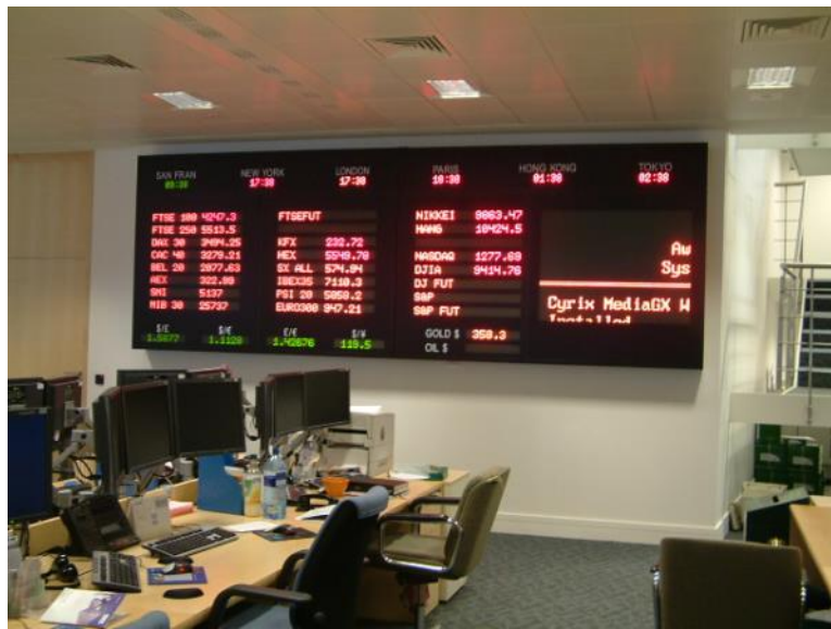
Left: 60mm Character Height single colour display (single colour LED boards using green and red) Trader stocks. Video board to right and global time zone clocks at the head of the board
