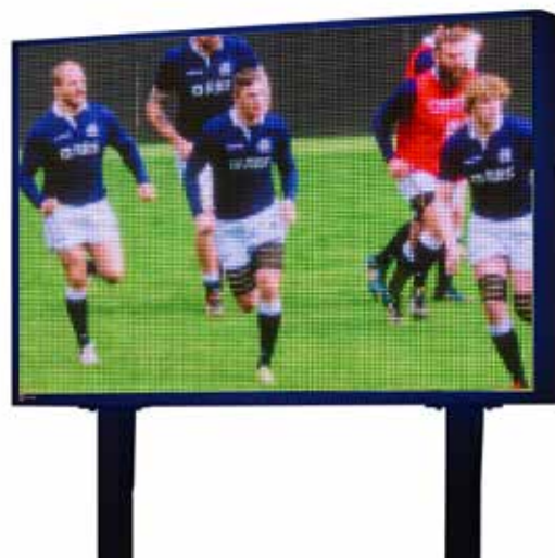
6.67mm pitch 150 x 100 resolution 100 x 667mm Viewed at 2 metres which is too close!
