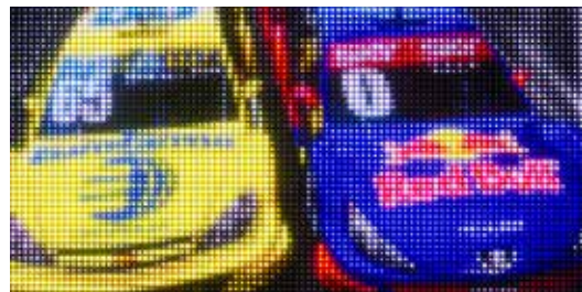
10mm pitch - 96 x 48 pixels viewing at 2 metres
