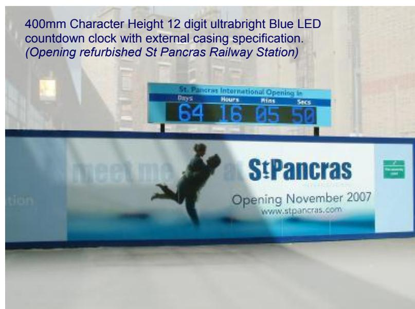
400mm Character Height 12 digit ultrabright Blue LED countdown clock with external casing specification. (Opening refurbished St Pancras Railway Station)
