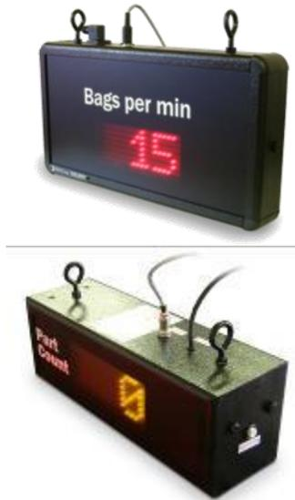
Above: Two simple double digit Counter displays, simple casing, top fixings
