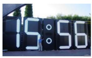
Above: 4metre electromechanical clock controlled by master clock controller
