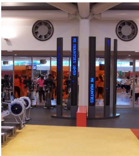
Left: Photo shows built in (bespoke) single line displays. Blue - 100mm character height Red - 60mm character height
