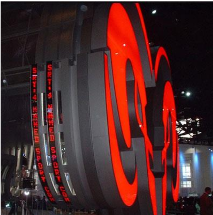
Left: Photo shows built in (bespoke) single line displays. Blue - 100mm character height Red - 60mm character height
