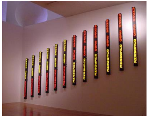
Left: Photo shows built in (bespoke) single line displays. Note the orientation of the characters in the red display and the slight curve to the display boards. Red - 60mm character height
