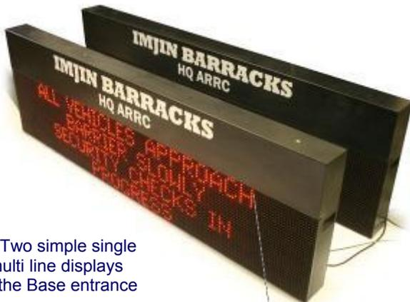
Above: Two simple single colour multi line displays used at the Base entrance
